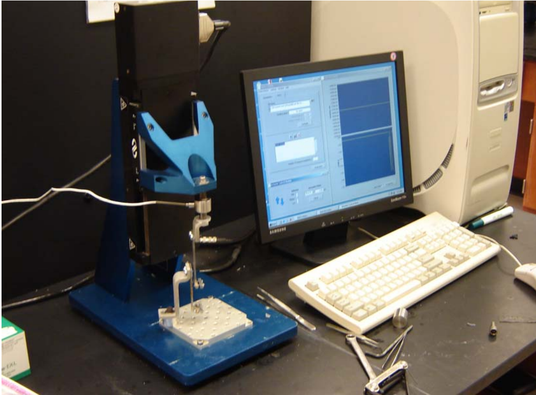
Figure 9 MACH1 micromechanical testing system used to evaluate the tensile strength of chitosan scaffolds.
